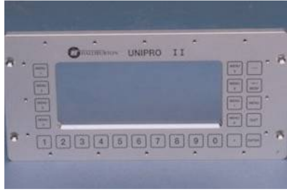
Control Panel for Cement Mixer
